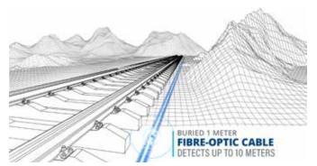
Each OptaSense solution is capable of protecting up to 40 killometers of track. Multiple systems can be linked to provide extended route coverage. The solution can be deployed on dedicated or existing fibreoptic cable. A site survey is required to confirm the viability of existing fiber-optic cable for rockfall and landslide detection.
