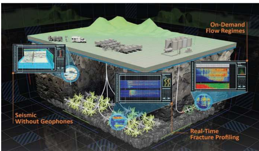
Figure 5. Distributed fibre optic sensing – well placement and completion design optimisation.
