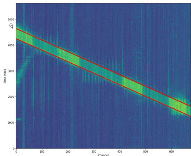
Figure 2 - Red lines indicate the front and back of the train to provide the ground truth information for the identified machine learning method.
