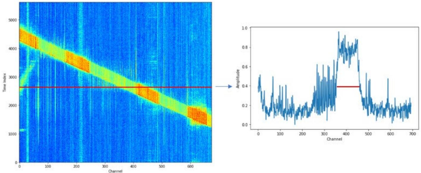
Figure 1 - (left) Fibre Sensing frequency band extracted data showing a train moving at constant speed. The higher-level red sections are where the train travels through a tunnel. The red line indicates the time index of the data (right). On the right hand chart the red line shows the train length.
