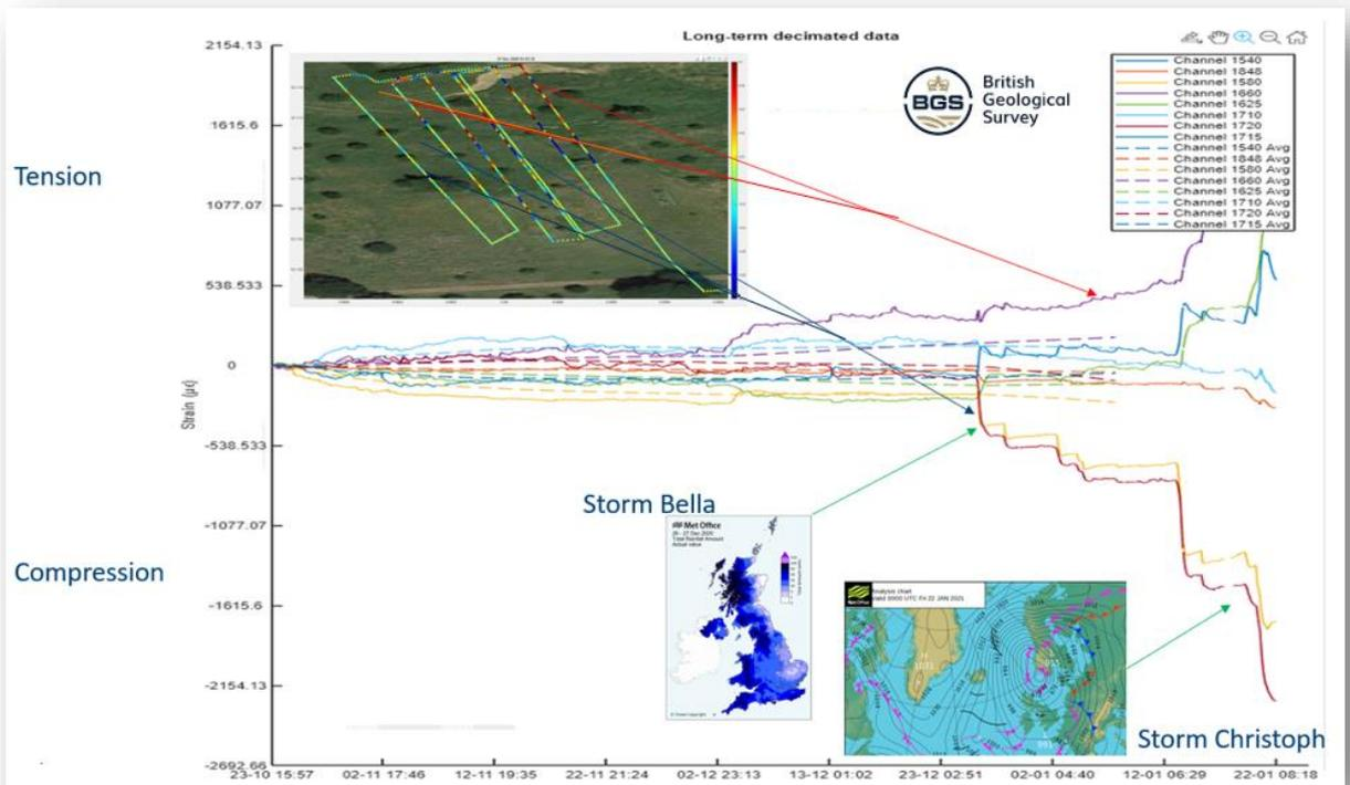
Monitoring the site over months allows you to look at both large scale features as we have here – large strains developing over months, punctuated by sharp transitions during bad weather.
