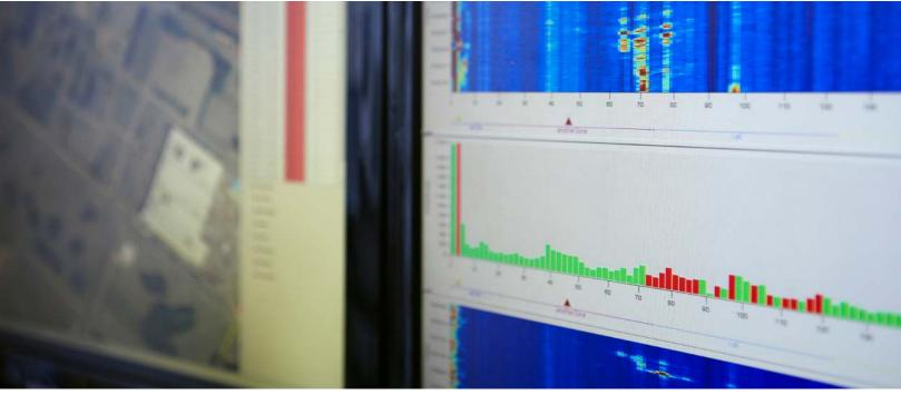
The OptaSense Perimeter Intrusion Detection System provides a visualization of any acoustic activity along the perimeter of the protected asset.
